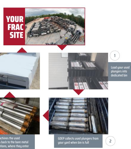
GDEP machines the used plungers back to the bare metal specifications, where they enter a proprietary coating process, and go through final machining to ensure quality OEM finish
