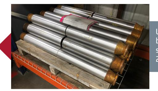
Used plungers are machined back to the bare metal specifications at GDEP's 20,000 sq. ft. facility
