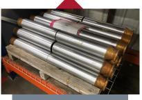
GDEP machines the used plungers back to the bare metal specifications, where they enter a proprietary coating process, and go through final machining to ensure quality OEM finish
