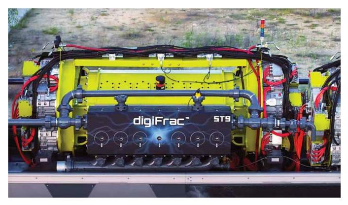
**Above:** To improve system durability, Liberty's digiFrac electric pump features a power frame with a curved internal geometry that the company believes will improve laminar flow and reduce the risk of cavitation.
