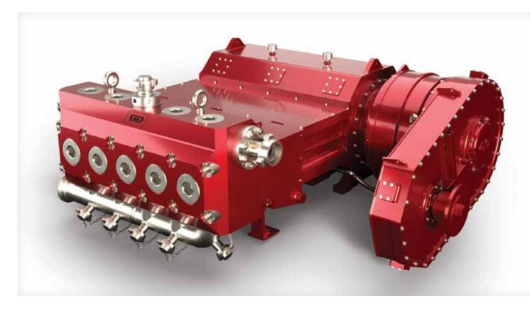
The Thunder 5000 HP Quintuplex Pump, the first 5,000-hp offering from GD Energy Products, can reduce the size of a frac spread by 30% compared with a 3,000-hp pump. To compensate for the increased stress that a 5,000-hp pump places on its components, the design features a longer stroke length and a harder lubricant to reduce scuffing and friction.
